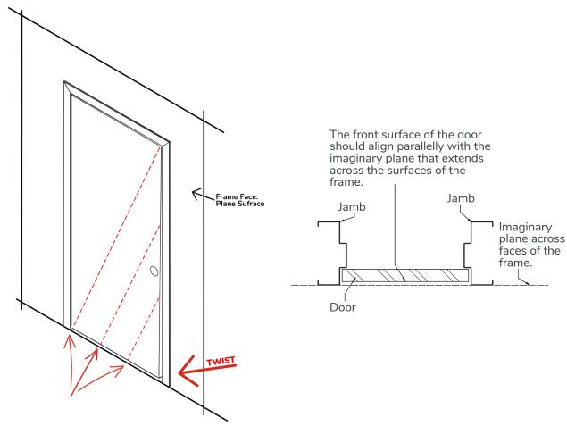
Door twists may appear in various positions depending on the door. Typically, it is observed diagonally, spanning between the lower and upper corners situated on opposite sides.
