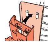
Before inserting the frame into the opening make sure your frame and adjustable expander sides are aligned.
