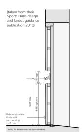
Sports hall walls should be detailed for safety and without hazardous projections. Flush surfaces should extend to 2.0m minimum, preferably to 2.7m above.
